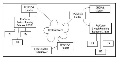
Figure 2-1. Dual-Stack ProCurve Switches Employed in an IPv4/IPv6 Network
